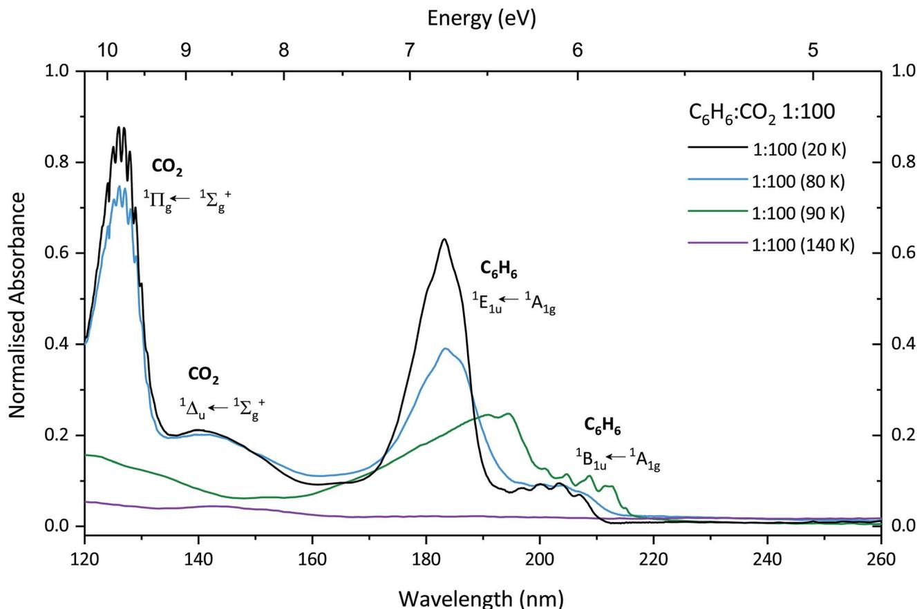
Fig. 2 VUV photoabsorption spectra of a 1 : 100  $C_6H_6 : CO_2$  mixture deposited at 20 K (black) and annealed to 80 K (blue), 90 K (green) and 140 K (purple). The spectra are normalised to the integrated area of the overlapping  ${}^1E_{1u} \leftarrow {}^1A_{1g}$  and  ${}^1B_{1u} \leftarrow {}^1A_{1g}$  transitions of the 1 : 100  $C_6H_6 : CO_2$  mixture deposited at 20 K.
