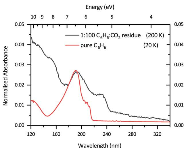
Fig. 4 VUV photoabsorption spectra of a 1 : 100  $\text{C}_6\text{H}_6$  :  $\text{CO}_2$  mixture which was irradiated with 1 keV electrons for 180 min and annealed to 200 K (black) to form a residue compared with pure benzene (red) at 20 K. The pure benzene spectrum at 20 K has been normalised to the peak height at  $\lambda = 190$  nm of the 1 : 100  $\text{C}_6\text{H}_6$  :  $\text{CO}_2$  residue.
