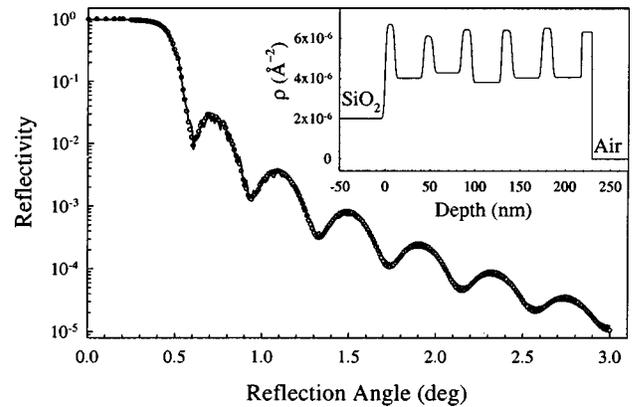
FIG. 1. Grazing incidence x-ray reflectivity (GIXRR) pattern for the  $\text{Co}_{10.0 \text{ nm}}/\text{Fe}_{30.0 \text{ nm}}$  multilayer (open circles: the experimental data, and continuous line: the best fit). The profile of the scattering length density  $\rho$  is also shown (inset).
