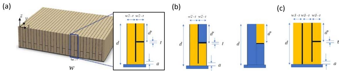
**Figure 6** (a) A partition configuration and inset with alternating hard-backed layer depths connected by a gap (b) hypothetical components of this cell type and (c) the configuration in (a) with an added hard-backed layer sub-cell.
