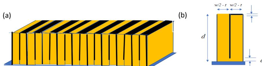
**Figure 5** (a) An arrangement of partitioned cells in a hard-backed layer of porous material
