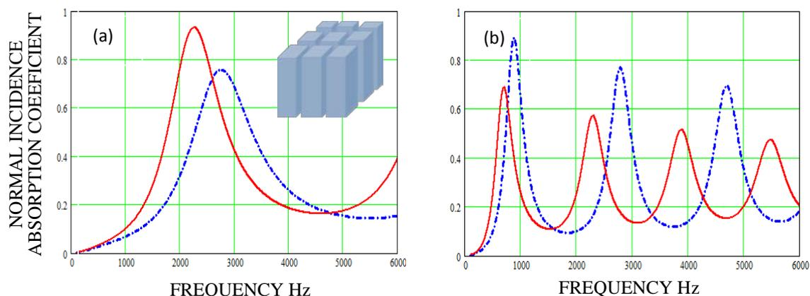
**Figure 4** Absorption coefficient spectra predicted for a 30 mm thick hard-backed layer, porosity 0.3, containing uniform 2 mm wide meso-slits and 0.2 mm wide micro-slits (broken blue lines) compared with those predicted for meso-slits with alternating 10 mm and 2 mm wide sections and 0.2 mm wide micro-slits (continuous red lines) (a) parallel to and (b) inclined at  $70^\circ$  to the surface normal.
