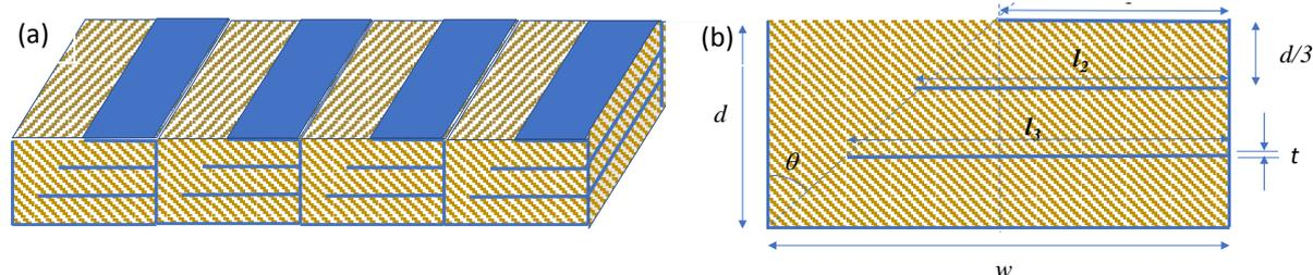
**Figure 8** (a) A porous layer of thickness  $d$  with vertical partitions between contiguous cells and horizontal partitions at different depths within each cell (b) a cell of width  $w$  with horizontal partitions spaced at  $d/3$  and with edge slope angle  $\theta$  of 30°
