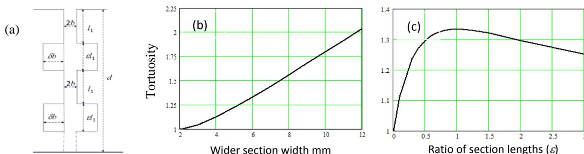
**Figure 2** (a) a periodically non-uniform slit; (b) and (c) predicted variations of tortuosity with the dimensions of the non-uniformity using eqn. (13a).
