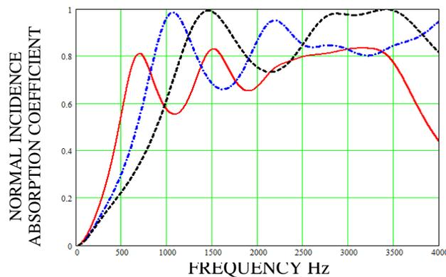
**Figure 11** Predicted influence of horizontal partition edge slope ( $33^\circ$  (broken black line),  $20^\circ$  (dash-dot blue line) and  $10^\circ$  (continuous red line)) on absorption spectra associated with 3 cm thick hard-backed partitioned inclined slit configurations other dimensions as for Fig. 10.
