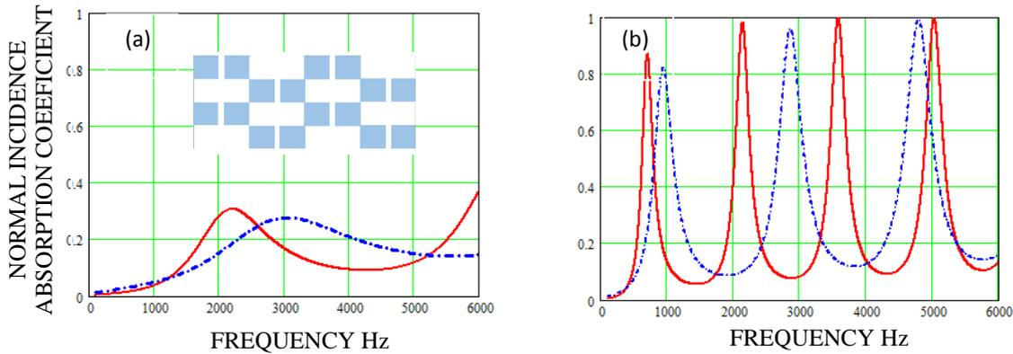
**Figure 3** Absorption coefficient spectra predicted for a 0.03 m thick hard-backed layer with porosity 0.6 containing uniform 1 mm wide slits (broken lines) separated by 0.67 mm compared with those predicted using (13) and (15) – (18) for staggered non-uniform pores with 1 mm wide narrow sections and 5 mm wide wider sections ( $\delta = 4$ ) of the same length ( $\varepsilon = 1$ ) (continuous lines): (a) parallel to the surface normal (b) inclined at  $70^\circ$  to the surface normal.
