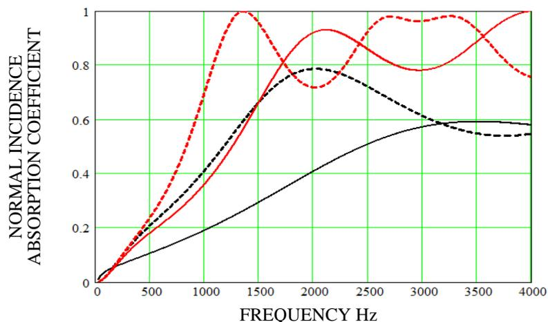
**Figure 9** Normal incidence absorption coefficient spectrum predicted for a metallic fibre material [4] (solid black line) and spectra predicted for an unpartitioned array of 0.28 mm wide slits inclined at 45° (broken black line) and for partitioned systems (Figure 9(a)) with slits either normal to the surface (solid red line) or inclined at 45° (broken red line)
