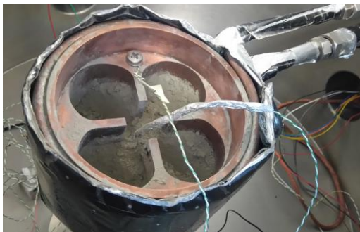
Figure 4 NU-LHT-2M sample held in the insulated copper container
