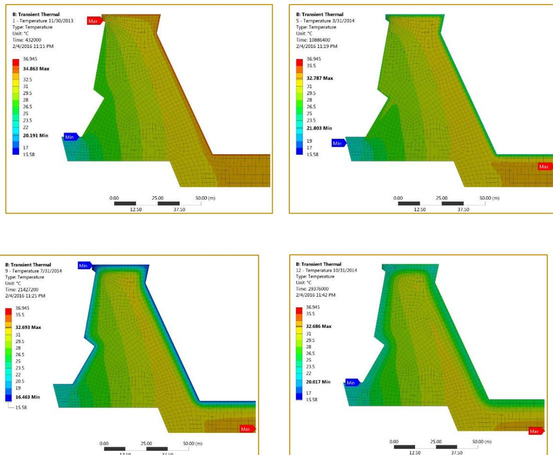
The color scale at the left hand side of each of the four diagrams in Figure 7 shows the various temperatures (in Celsius) in increasing order from minimum values at the bottom (dark blue) to maximum values at the top (red). Looking at the block in each diagram, note that the highest temperatures are in the downstream phase (contact with the environment), while warmer temperatures are located upstream (contact with the reservoir).
