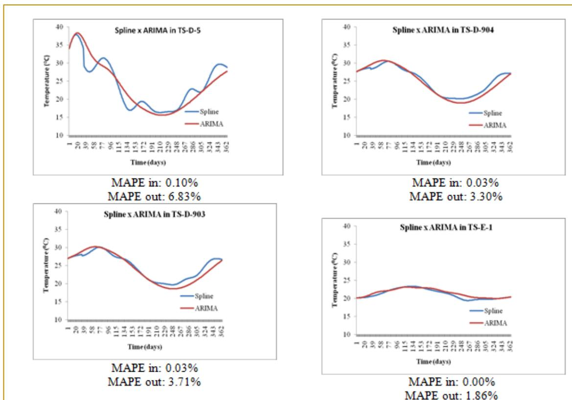
Note from the plots in Figure 6 and the respective low MAPE in values that the forecasts by the ARIMA models are approximating well the data interpolated by cubic splines.
