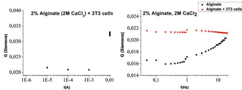
**Figure 9.** Conductance of 2% (w/v) NaAlg HGs crosslinked with Ca<sup>2+</sup> at 2M, containing S-DMEM and 3T3 fibroblasts, (left) as a function of current intensity, at an AC frequency of 10 Hz: (right) as a function of AC frequency, at a current intensity of  $10^{-4}$  A.
