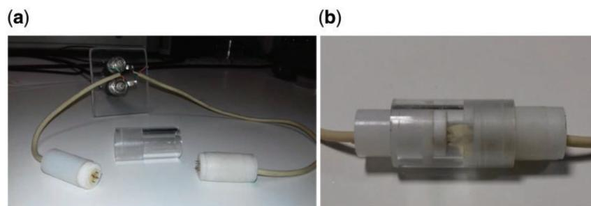
**Figure 3.** Detailed view of the four-point-probe and cylindrical sheath: (a) 10 stainless steel electrodes, the external electrodes provide current, whereas the central electrodes measure the voltage; the sheath minimises dehydration losses; (b) alginate hydrogel (with lateral dimensions 10 mm × 15 mm) placed in the R-cell prior to measurement.
