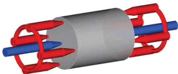
**Figure 2.** The four-probe setup realised in this work. The central electrodes (marked with blue) are the sense electrodes to measure sample voltage. The red electrodes are the force electrodes (multiple on each side) to apply the stimuli in a uniform manner. The grey cylindrical shape corresponds to the actual sample being measured.
