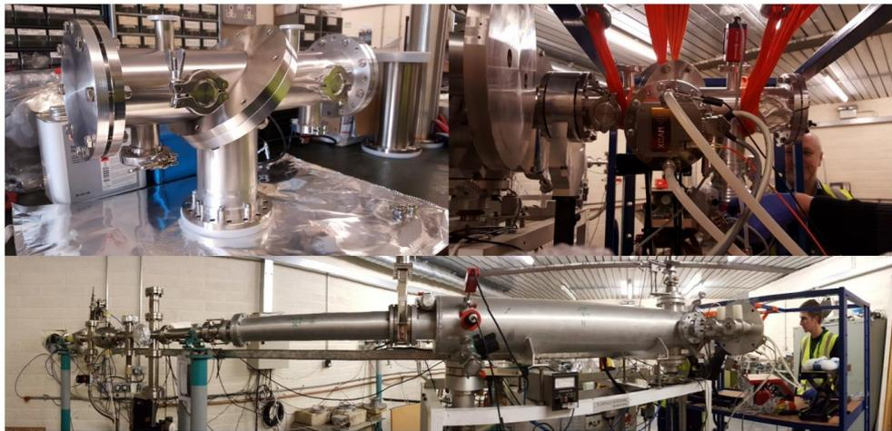
**Figure 4.** Experimental equipment for tests performed during campaign 1 at the Synergy Health proton facility at Harwell, UK (~6 MeV).
