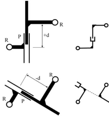
**Figure 3.** Positive and negative distance for a prismatic joint, and a schematic representation
