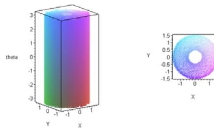
**Figure 5.** Workspace of the RRR planar serial manipulator.
