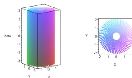
**Figure 7.** Workspace of the RPR planar serial manipulator.
