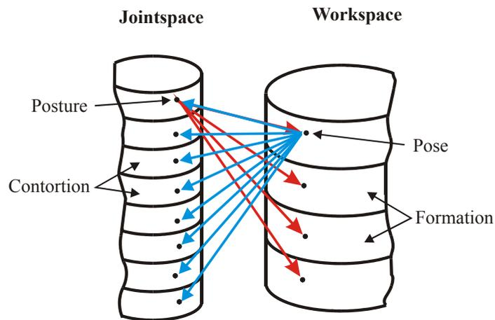
**Figure 1.** Mapping between the joint space and the workspace.
