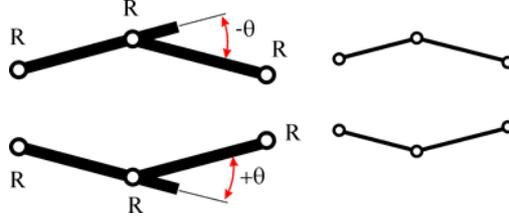
**Figure 2.** Positive and negative angle for a revolute joint, and a schematic representation.
