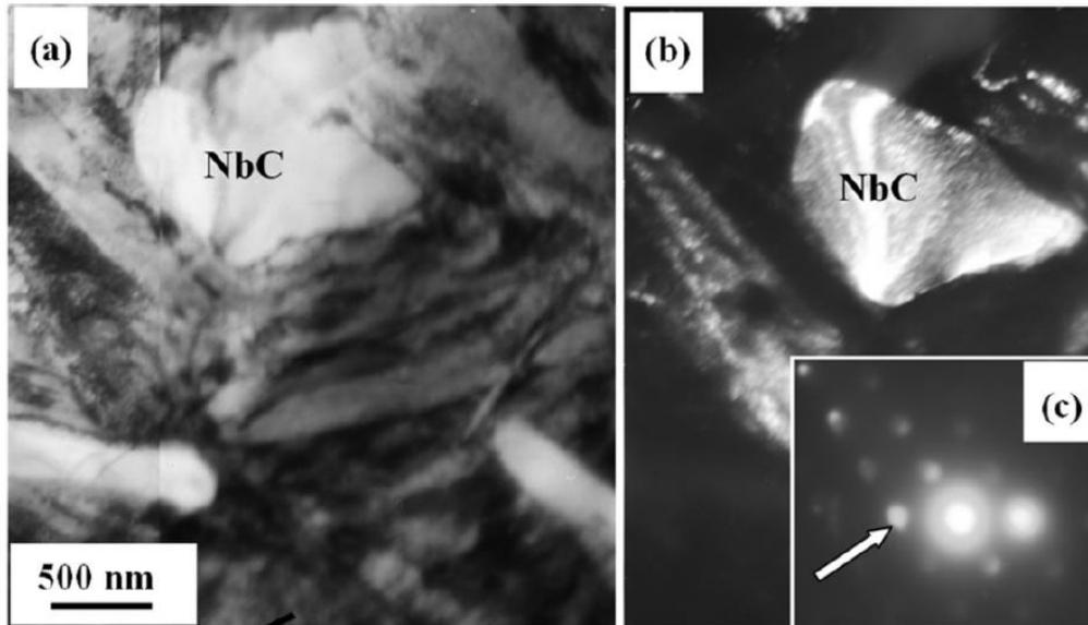
Fig. 4. Electron microscope image of surfacing structure applied with wire №1 on Hardox 450 steel; a – light field; b – dark field obtained in closely located reflections  $[002] \text{NbC} + [110] \alpha\text{-Fe}$  (the reflections are designated with arrow in (c)); c – micro-electron diffraction pattern, the arrow designates the reflections in which dark field was obtained.
