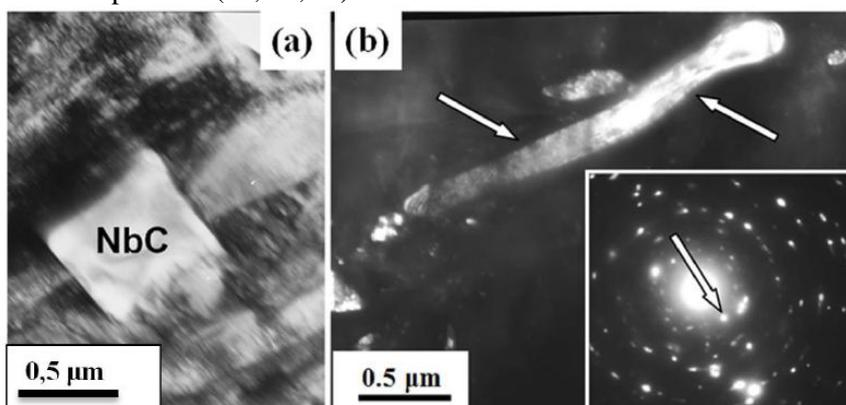
Fig. 3. Electron microscope image of surfacing structure applied with wire №1 on Hardox 450 steel; a – light field; b – dark field obtained in reflection [002] NbC (it is designated by the arrow in micro-electron diffraction pattern). In (b) niobium carbide is designated by arrows.
