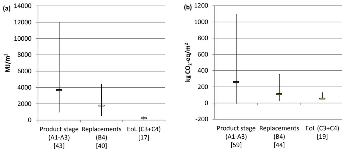
Figure 2. EE (a) and EG (b) averages and ranges from selected reported life cycle stages. Square brackets indicate number of case studies included in the displayed ranges
