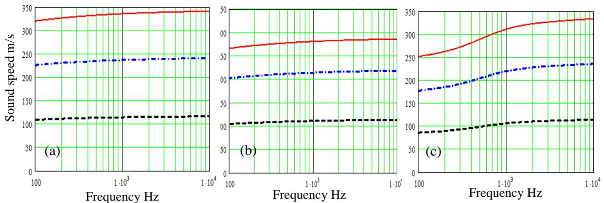
**Figure 10** (color online) Predicted dispersion of sound in a rigid-porous medium (porosity 0.3) with slits inclined to the surface normal at 0° (continuous red lines), 45° (dash-dot blue lines) and 70° (broken black lines) assuming (a) uniform 2 mm wide slits (b) sinusoidally-varying widths, wavelength 0.3 mm, amplitude 0.2 mm (outer width 2 mm) and (c) dual-porosity with meso- (2mm wide, edge-to-edge spacing 8 mm) and micro-slits (0.2 mm wide, edge-to-edge spacing 1.4 mm).
