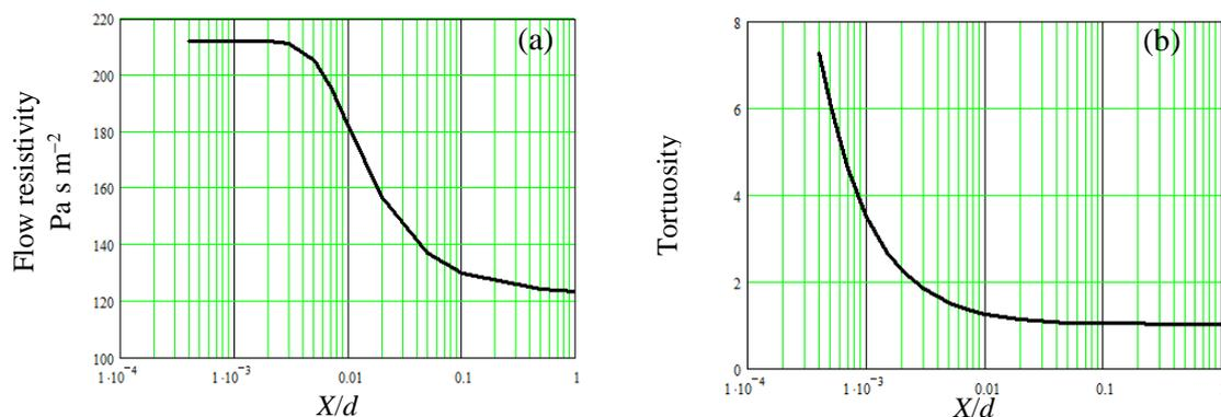
**Figure 7** Predicted influence of the fractional wavelength  $X/d$  of sinusoidal variation (amplitude 0.2 mm) in pore width on (a) flow resistivity and (b) tortuosity according to equations (19) and (20).
