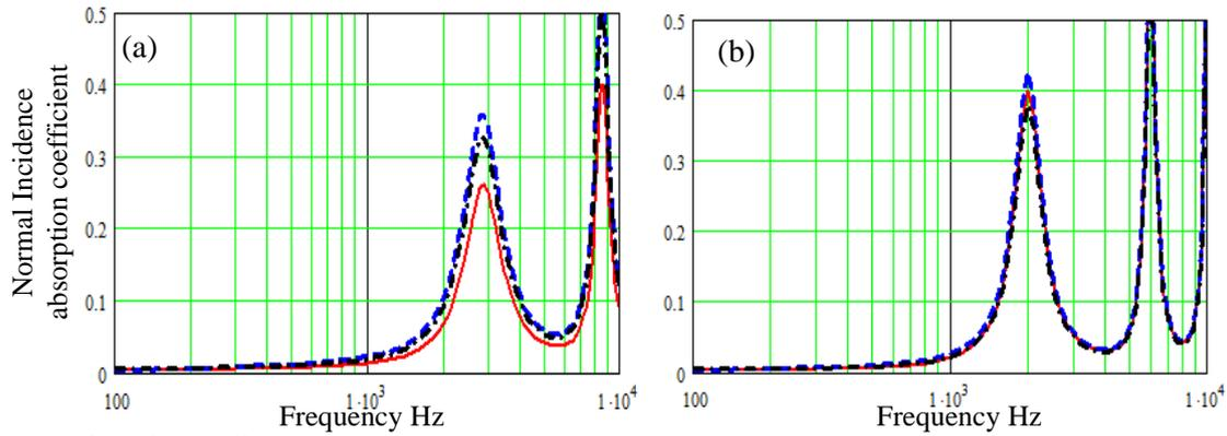
**Figure 6** (color online) Absorption coefficient spectra predicted for a 3-cm thick hard-backed rigid porous layer with porosity 0.3 containing identical parallel 2 mm wide slits (continuous red lines), or log-normal width distributions (standard deviation  $0.5 \phi$ -units) of uniform slits (broken blue lines) or of non-uniform slits (dash-dot black lines) (a) parallel to the surface normal and (b) inclined at an angle of  $45^\circ$  to the surface normal.
