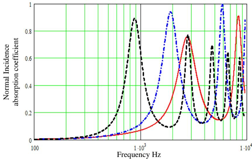
**Figure 9** (color online) Predicted absorption coefficient spectra for a 3-cm thick hard-backed rigid-porous layer containing a microstructure of 2 mm wide meso-slits, edge-to-edge spacing 8 mm and 0.2 mm wide micro-slits, edge-to-edge spacing 1.4 mm, parallel to the surface normal (continuous red line) or at 45° to the surface normal (dash-dot blue line) or at 70° to the surface normal (broken black line).
