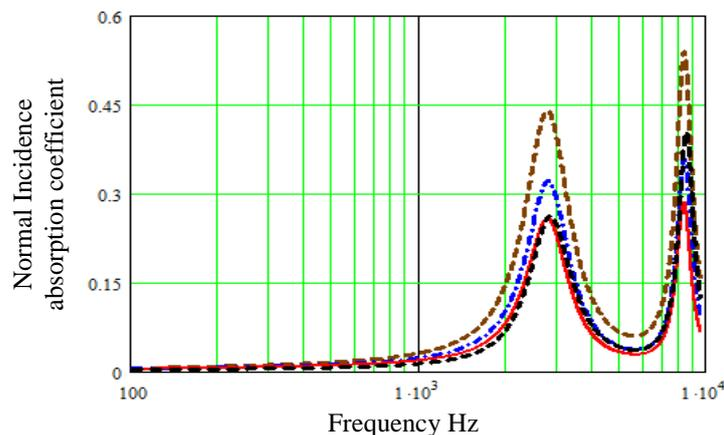
**Figure 3** (color online) Absorption coefficient spectra predicted for a 0.03 m thick hard-backed rigid-porous layer with porosity 0.3 containing (normal to the surface) parallel 2 mm side identical square pores (broken brown line), 2 mm wide slit pores (continuous red line) and rectangular pores with longer sides of 4 mm (dash-dot blue line) and 8 mm (broken black line).
