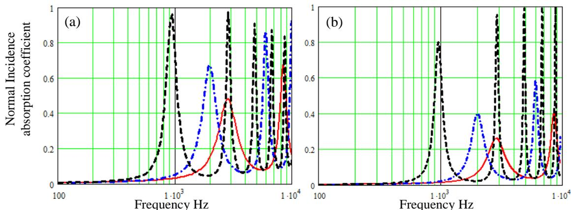
**Figure 2** (color online) Predicted absorption coefficient spectra for 0.03 m thick rigid-porous layers with porosity 0.3 containing parallel uniform identical pores at angles to the surface normal of  $0^\circ$  (continuous red lines),  $45^\circ$  (dash-dot blue lines) and  $70^\circ$  (broken black lines): (a) cylindrical pores radius 1 mm and (b) slit pores width 2 mm.
