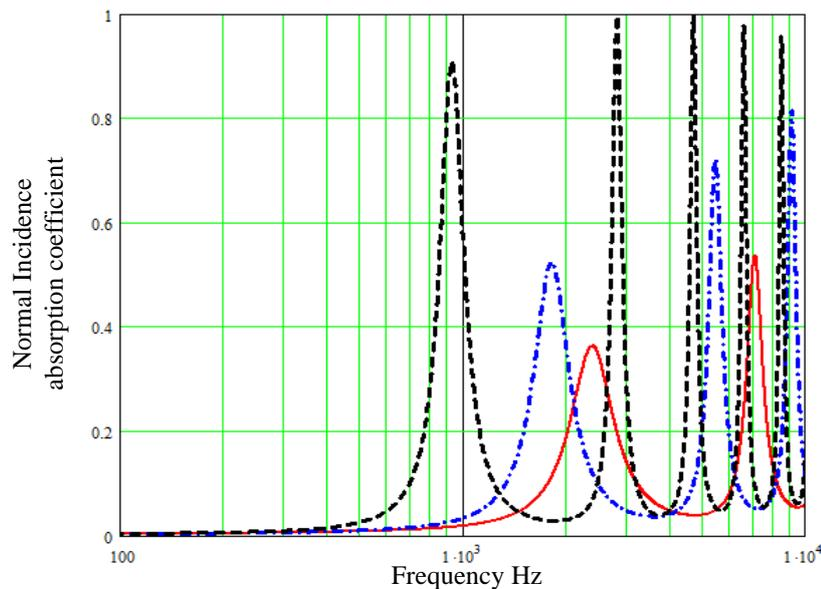
**Figure 8** (color online) Predicted absorption coefficient spectra for a 3-cm thick hard-backed rigid porous layer containing parallel slits with a sinusoidal width variation (amplitude 0.2 mm, wavelength 0.024 mm, outer width 2 mm, edge-to-edge spacing 2 mm) normal to the surface (solid red line), inclined at  $45^\circ$  (dash-dot blue line) and inclined at  $70^\circ$  (broken black line).
