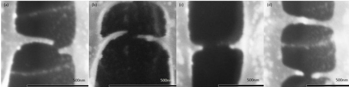
**Figure 1.** SEM images of nanowire bridges (NWBs) after fracture. (a) 30 nm radius: flat-ended cantilevers formed; (b) 20 nm radius: tapered cantilevers formed; (c) 8 nm radius: cantilever retraction and bulbous ends formed; (d) 8 nm radius: bulbous ends on both sets of cantilevers. Retraction is observed only on the lower NWB; the upper NWB has reformed from recoiling cantilevers (see below). Not possible to change scale indicators
