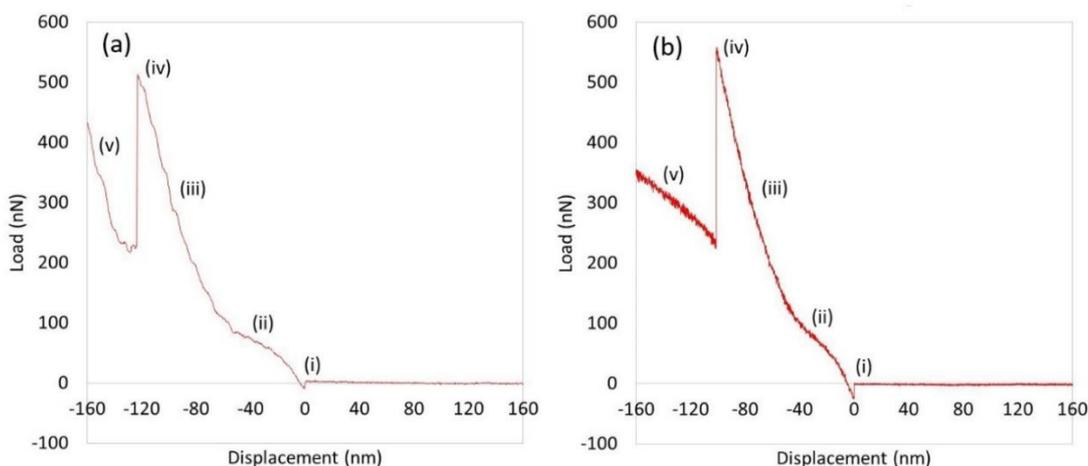
**Figure 2.** AFM load-displacement data showing mid-point loading. (a) Nanowire bridge of radius 30 nm: fracture occurs at a mid-point load of 512 nN (b) Nanowire bridge of radius 8 nm: fracture occurs at a mid-point load of 556 nN.
