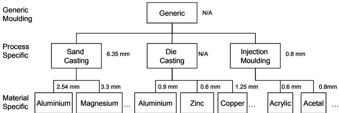
Figure 2. Sample Facts Hierarchy for Minimum Wall Thickness
