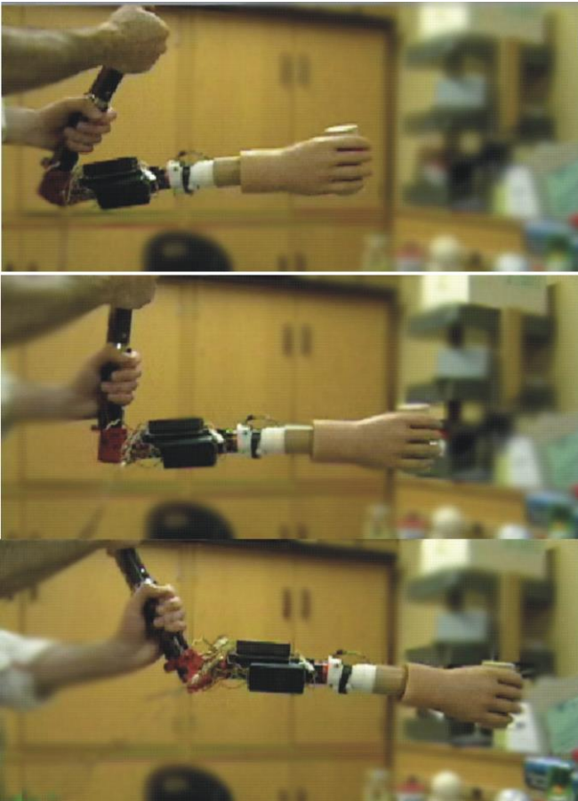
Fig. 9. Motion Compensation - The humeral section flexes and extends and the motion is detected by the accelerometers in the wrist and the elbow is driven to compensate for the motion.
