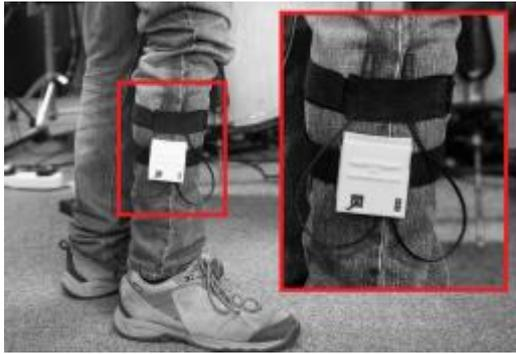
Fig. 1 The Haptic Bracelet device fitted on user's leg
