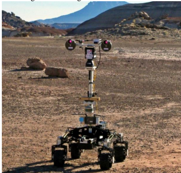
Fig. 1. MURFI 2016 Rover. The large “eyes” contain the PanCam filter wheels.
