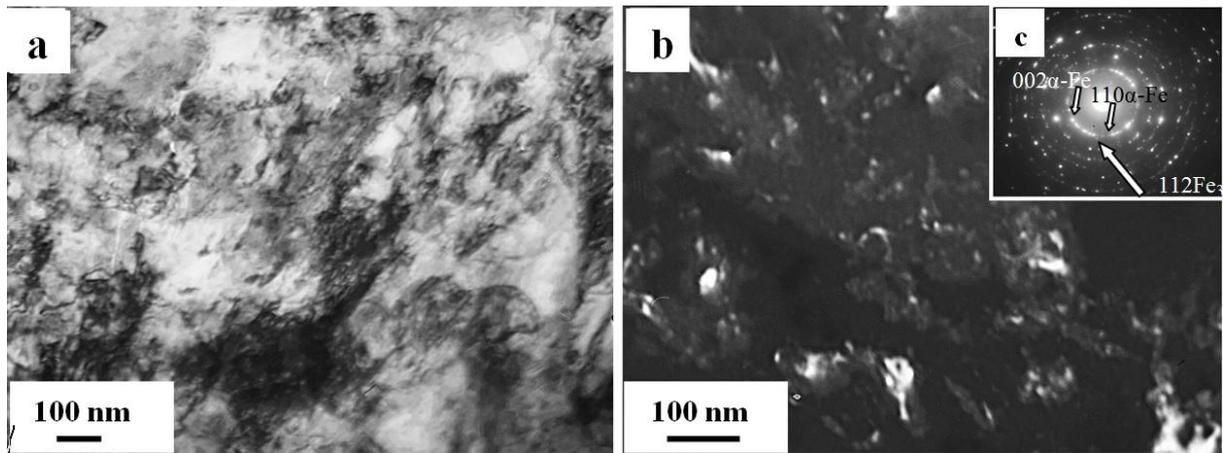
**Figure 4.** TEM images reveal the microstructure in surface layer of rail steel after 500 MTGW loading. (a) light field; (b) dark field obtained in reflection  $[112] \text{Fe}_3\text{C}$ ; (c) micro-electron diffraction pattern, arrow designates the reflection in which dark field was obtained.
