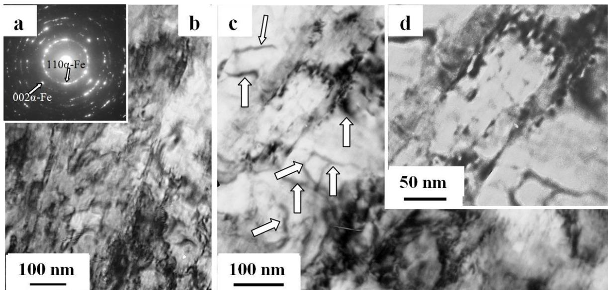
**Figure 5.** SEM and TEM image for the surface layer of steel after 500 MTGW loading. (a) diffraction patten from (b); (b)-(d) are the light field images.
