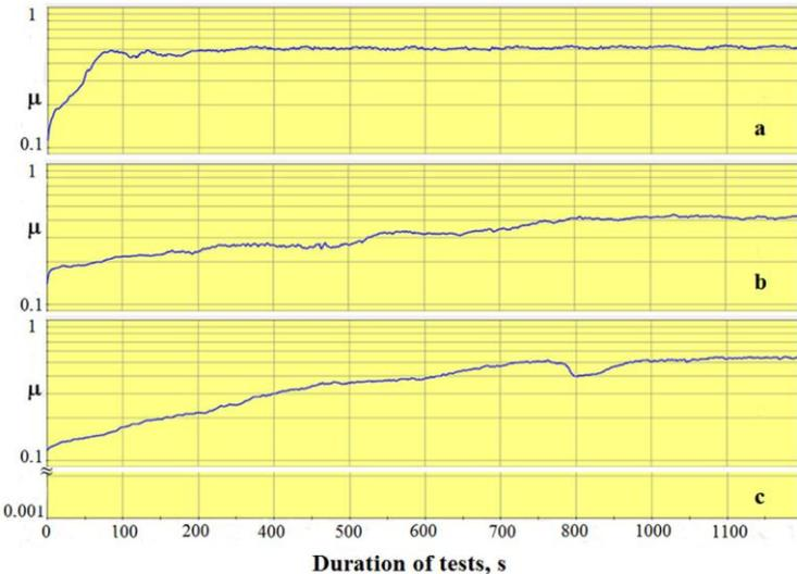
**Figure 2.** The change of friction coefficient  $\mu$  for (a) new steel, (b) steel after 500 MTGW loading, and (c) steel after 1000 MTGW loading. The wear resistance tests were done on rail tread surface.
