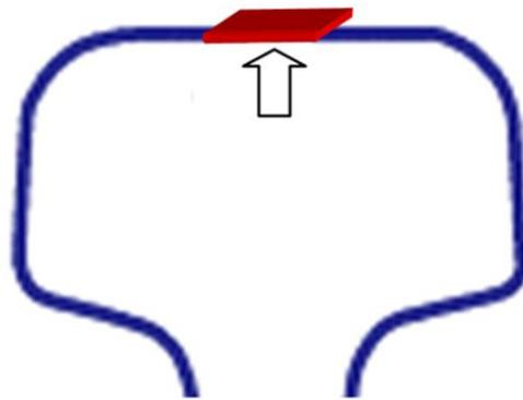
**Figure 1.** Schematic diagram shows the samples position (where an arrow is pointing to) in rail steel.
