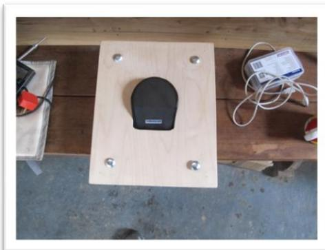
Figure 5: Button made from sewing machine pedal
