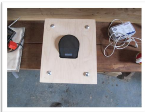
Figure 5: Button made from sewing machine pedal
