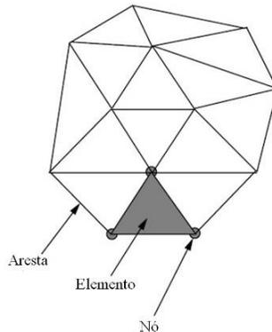
**Figure 3.** Exemple of finite element mesh.
