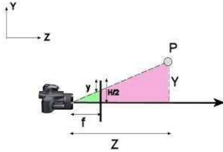
Fig. 6. Side view of the side-by-side camera pair
