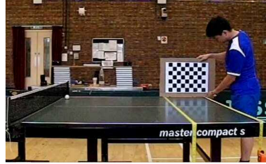
Fig. 7. A upright double-sided checkerboard was used for creating reference points.
