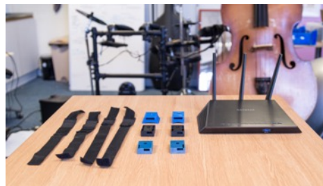
Fig. 2. The Haptic Bracelets (middle) with Velcro straps (left) and router (right)
