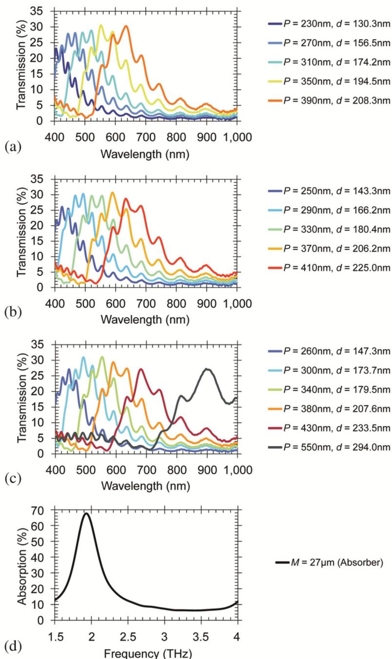
**Figure 3.** Measured spectral characteristics of the synthetic multispectral material (SMM). The transmission spectra associated with the plasmonic filters are shown in (a)–(c). The hole period,  $P$ , and hole diameters,  $d$ , as measured using the scanning electron microscope (SEM) are shown in the legend. (d) Absorption spectrum of the terahertz (THz) metamaterial (MM) component of the SMM.  $M$  is the period of the MM absorber unit cell.
