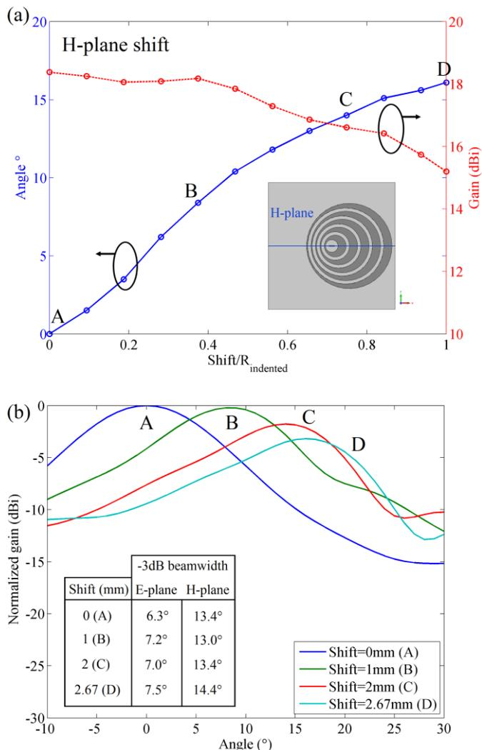
Fig. 6. Simulated angle ( $^\circ$ ) and gain (dBi) of the main beam according to the shift of the centre of the rings along the E-plane (a), and normalized radiation patterns for different values of Shift (0, 1, 2 and 2.67mm) (b); Inset table: 3dB beamwidths for E- and H-plane patterns shown in Fig. 5 (b) and Fig. 6 (b)
