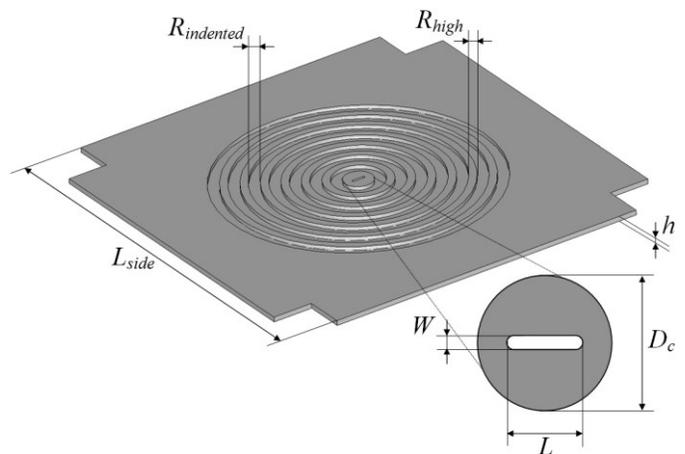
Fig. 1. Dimensions of the “Bull's eye” antenna
