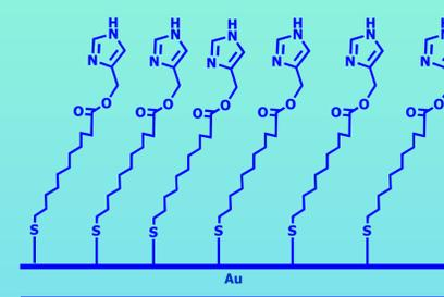
**Figure 4.** Imidazole/disulfide SAM on gold surface
