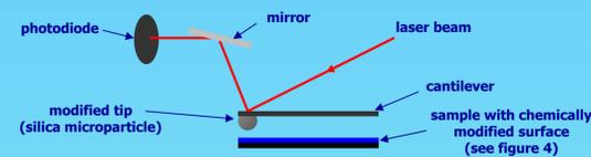
**Figure 1.** Measuring surface interactions using AFM
