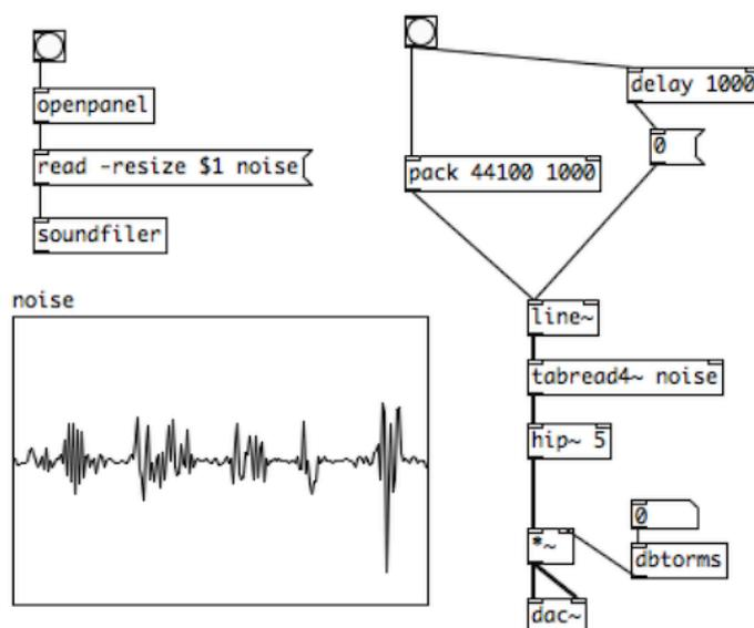
Image 2 - Sample playback in Pure Data, displaying a close mapping between the interface and the task being performed by the software
