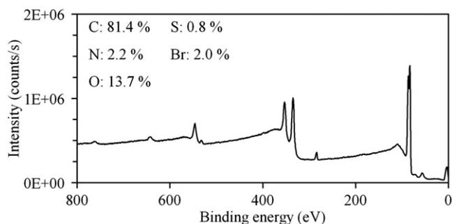
Fig. A3. XPS survey spectrum for SAM 3.
