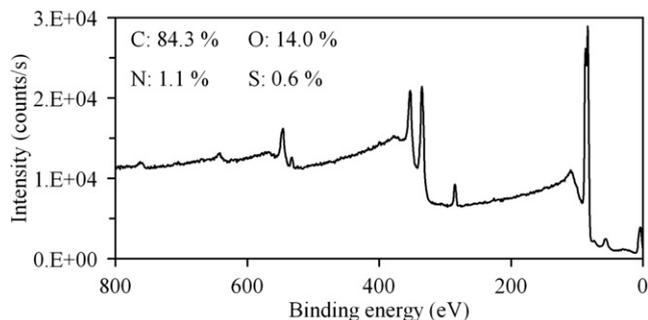
Fig. A4. XPS survey spectrum for SAM 4.
