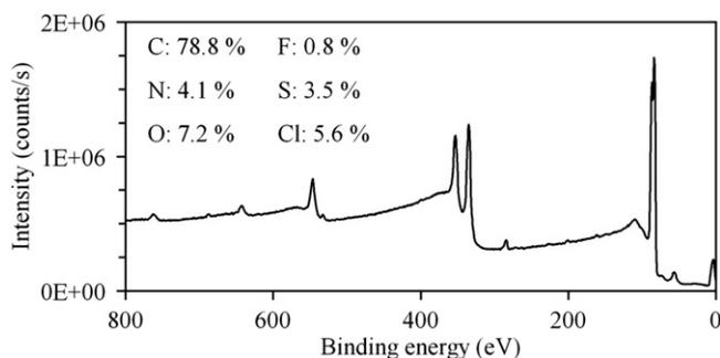
Fig. A1. XPS survey spectrum for SAM 1.
