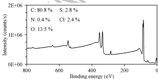
Fig. A2. XPS survey spectrum for SAM 2.
