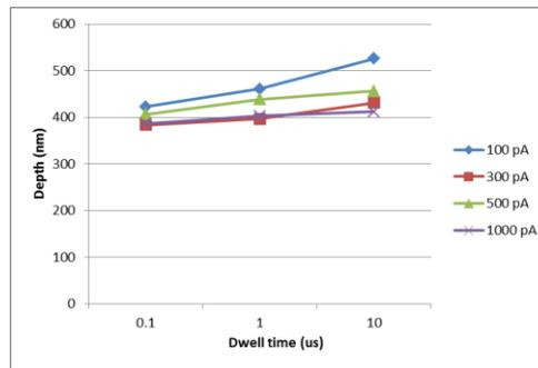
**Figure 3.** Effect of dwell time on milling depth at milling currents in the range 100-1,000pA
