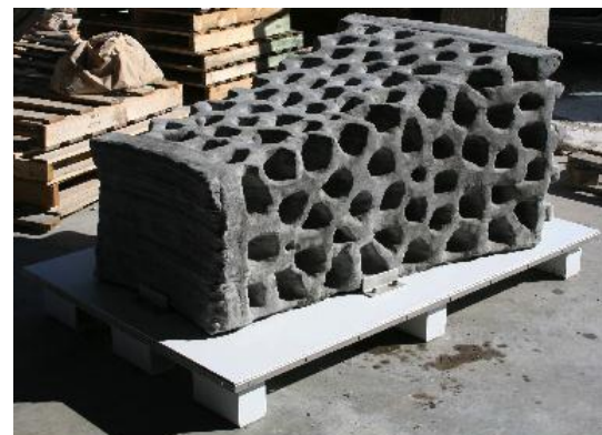
Figure 1: Printed block using a Lunar simulant (D-Shape) [22]. The approximate footprint of the block is less than 1,000 by 2,000 mm.
