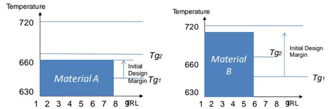
**Figure 4 Technology readiness and temperature at the beginning of the process**
