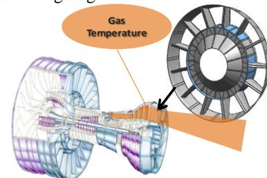
**Figure 3 A rear turbine structure of a jet engine exposed to hot gases**
