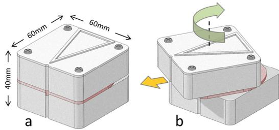
Figure 2: The Animotus a) in home pose, b) illustrating rotation and linear extension. These DOF may be individually actuated.
