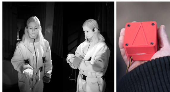
Figure 1: (Left) Audience members equipped with localization equipment, bone conducting headphones and *Animotus* (right)
