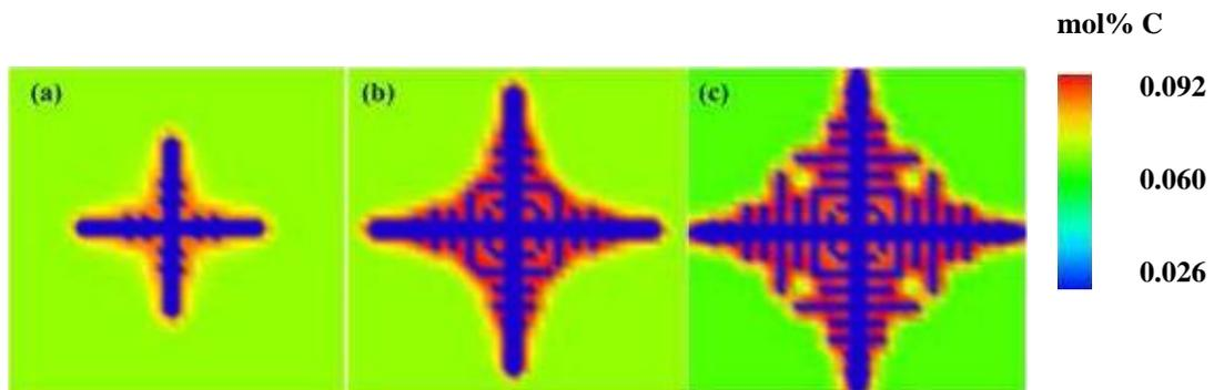
Fig.2. The carbon concentration profile of the equiaxed dendrite at  $t = 0.01s$  growing
