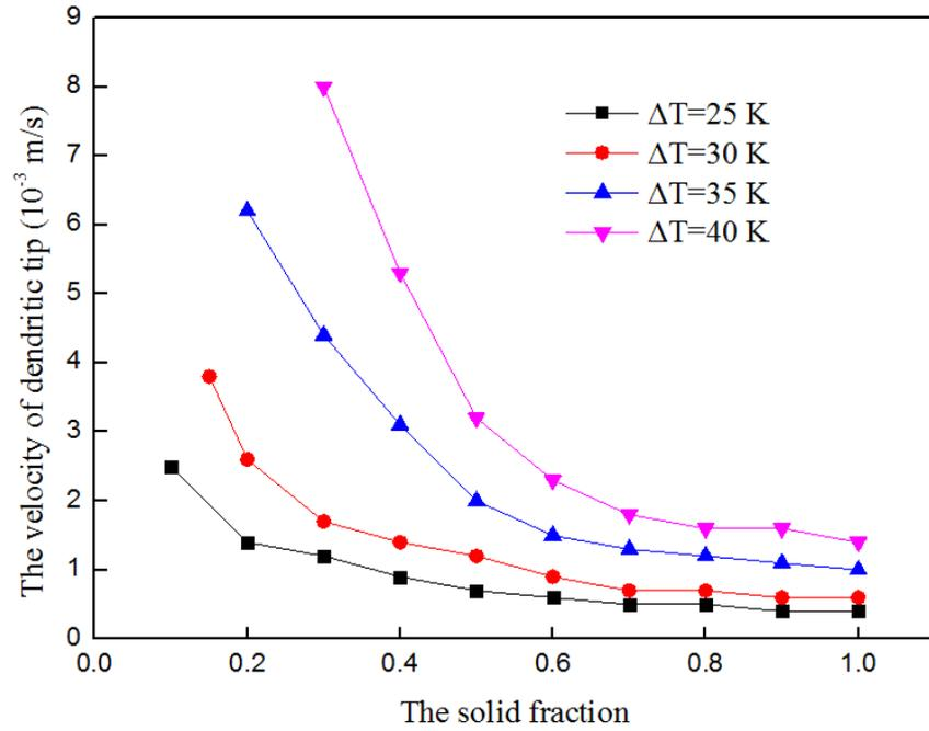
Fig.3. The velocity of the dendrite tip at  $t=0.01s$  as a function of the solid fraction at various undercoolings.
