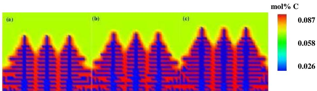
Fig.6. The carbon concentration profile at  $t = 0.036$  s with the convective heat transfer coefficient of (a)  $h = 1000 \text{ W m}^{-2} \text{ K}^{-1}$  ; (b)  $h = 1100 \text{ W m}^{-2} \text{ K}^{-1}$  ; and (c)  $h = 1200 \text{ W m}^{-2} \text{ K}^{-1}$  .
