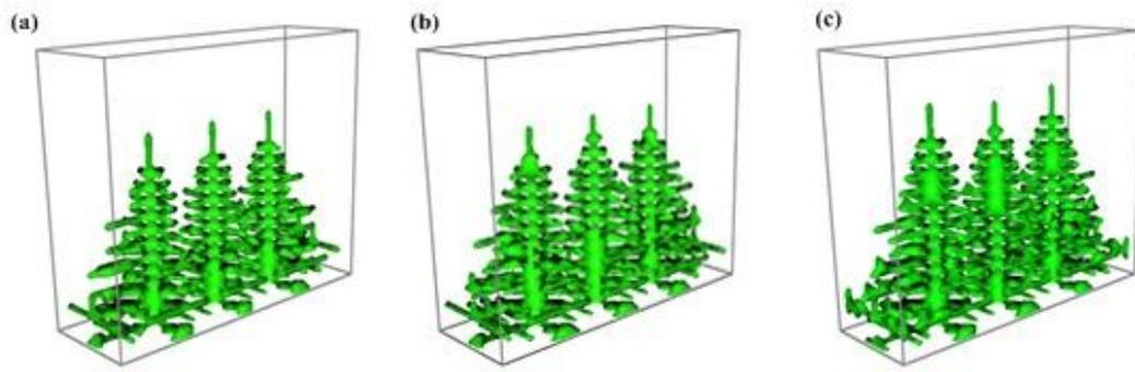
Fig.5. The dendrite morphology at  $t = 0.036$  s growing with the convective heat transfer coefficient of (a)  $h = 1000 \text{ W m}^{-2} \text{ K}^{-1}$  ; (b)  $h = 1100 \text{ W m}^{-2} \text{ K}^{-1}$  ; and (c)  $h = 1200 \text{ W m}^{-2} \text{ K}^{-1}$  .
