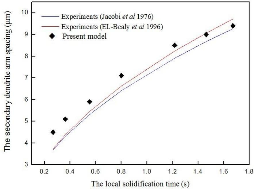
Fig.9 The dendrite secondary arm spacing vs. the local solidification time in directional solidification.
