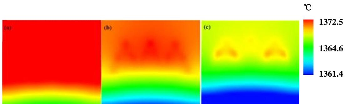
Fig.7. The temperature distribution at  $t = 0.036$  s with the convective heat transfer
