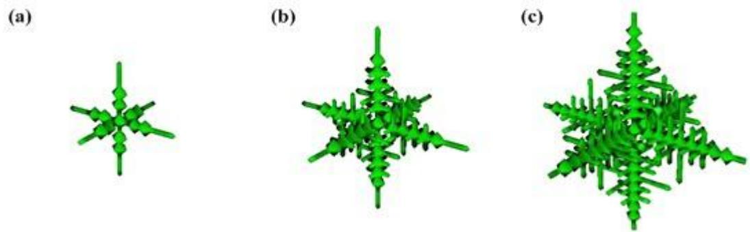
Fig.1. The morphology of the equiaxed dendrite at  $t = 0.01s$  growing at an undercooling of (a)  $\Delta T = 50K$  ; (b)  $\Delta T = 60K$  ; and (c)  $\Delta T = 70K$  .
