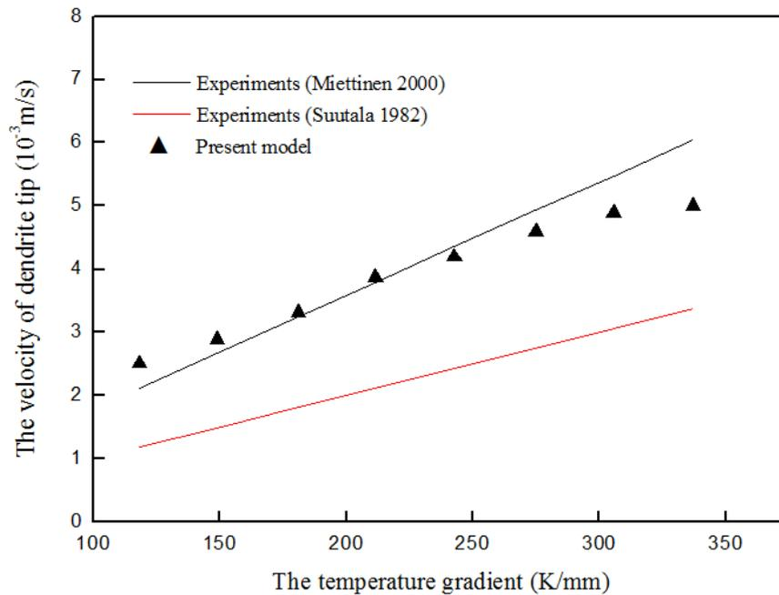
Fig.8 The velocity of the dendrite tip vs. the temperature gradient in directional solidification.
