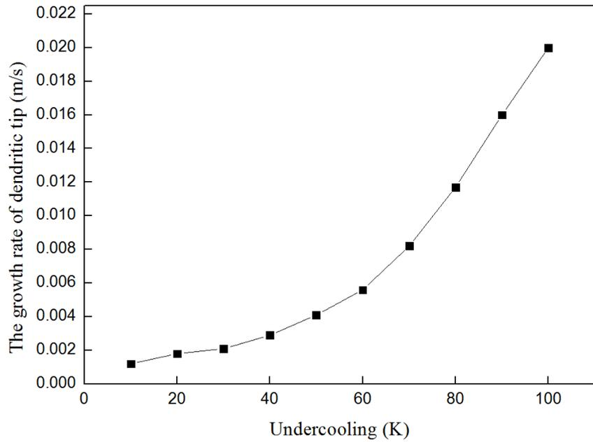
Fig.4. The average velocity of the dendrite tip at  $t = 0.01s$  at various undercoolings.
