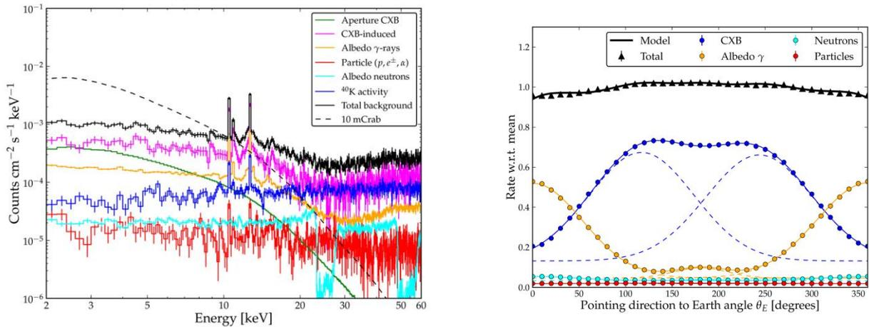
Figure 7: the background estimation for the LAD experiment, as derived by a detailed Monte Carlo simulation including a full geometrical description. *Left*: The black solid line shows the total background (sum of all components). The dashed line reports the energy-dependent requirement. *Right*: the orbital modulation of the total background rate (black line) and the individual components.
