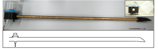
Figure 2: Top : Simplified bass clarinet (a cylindrical tube with a bass clarinet mouthpiece and a reed) with embedded control system with collocated microphone and speaker. Top right corner : control system removed from the instrument. Bottom : Schematic view of the instrument with embedded control system.
