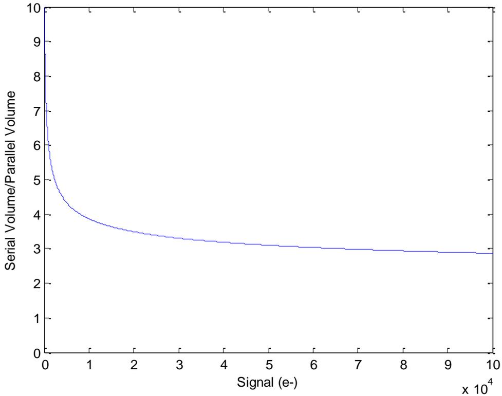
Figure 3: Difference between the volume of the charge packet calculated between the parallel and serial registers of the CCD204. These have a  $\sim 3x$  difference in active electrode area, but the charge packet volume actually varies depending on signal level and structure size, so only tends towards a  $\sim 3x$  difference at large signal levels.
