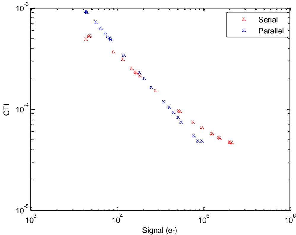
Figure 8: Charge transfer inefficiency calculated using the EPER technique from flat fields over a range of signal sizes. CTI is very high at small signal before reducing to an approximately constant value for large signals.
