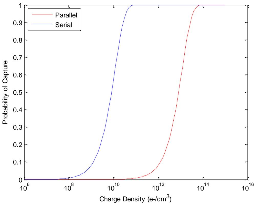
Figure 1: Trapping probability calculated for the PV centre trap ( $\sigma=5 \times 10^{-15} \text{ cm}^2$ ) depending on the charge dwell time/trap energy. Dwell times of  $t=1 \times 10^{-3} \text{ s}$  and  $t=1 \times 10^{-6} \text{ s}$  are plotted to reflect the readout speeds of the parallel and serial registers.
