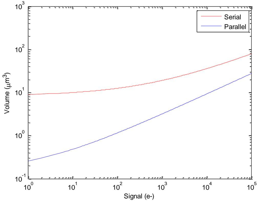
Figure 2: Comparison of the fit-lines which describe the signal-volume relationship calculated from device simulations of both the parallel and serial registers presented by Clarke 2012<sup>7</sup>. These take into account the difference in trapping probability between the two structures.
