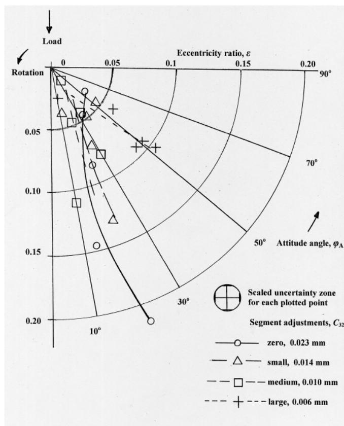
Fig 5 Static locus plots for different adjustments, 3500 rpm
