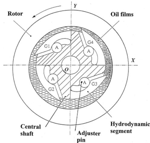
**Fig 2 – Cross section scheme of adjustable hydrodynamic segments**
