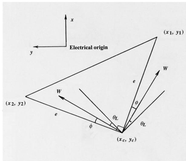
**Fig 3 – Shaft centre and rotor eccentricity**
