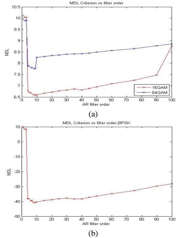
Figure 3. Effect of AR filter order on MDL in (4) for (a) 16QAM and 64QAM and (b) BPSK
