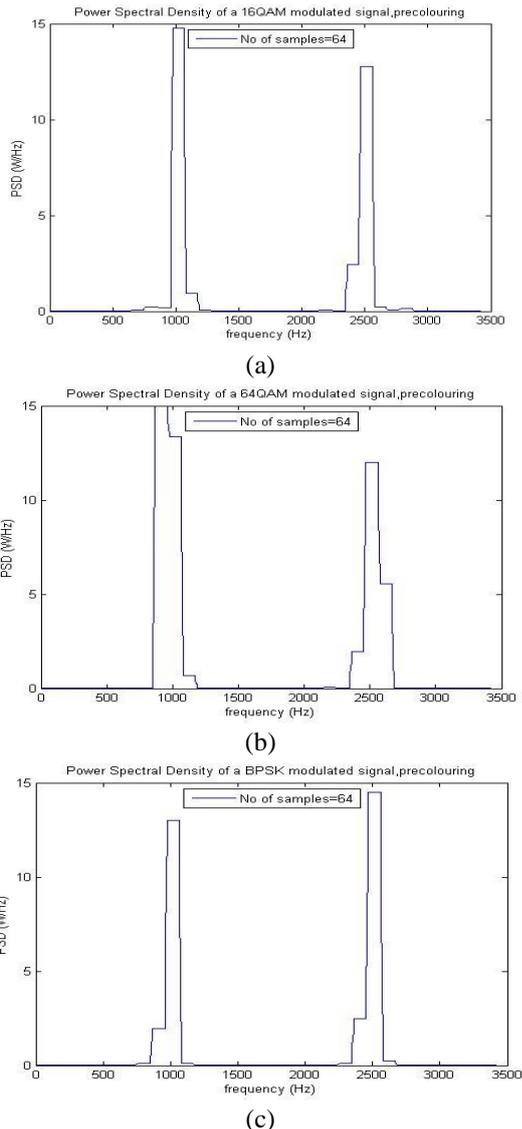
Figure 8. Recovered normalised PSD at sampling rates 4.25% Nyquist with precoloring for (a) 16QAM, (b) 64QAM and (c) BPSK
