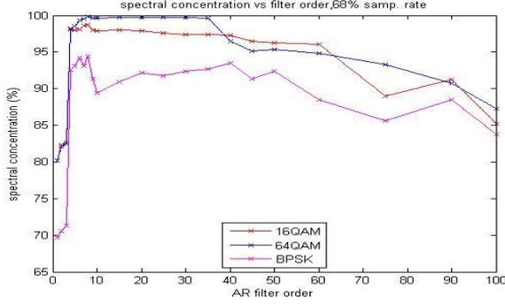
Figure 4. The effect of AR filter order on *PSD* spectral concentration
