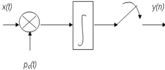
Figure 1. Block Diagram of the Random Demodulator (RD)
