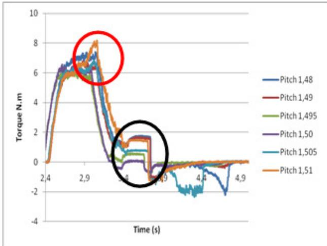
Fig. 6. Torque signal for tapping operation of AISI 1045 carbon steel at cutting speed of 30 m/min.
