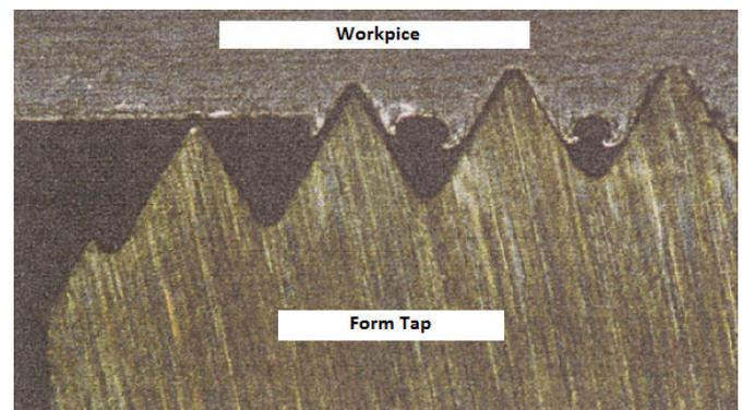
Fig. 1. Thread forming operation and the split crest [5].
