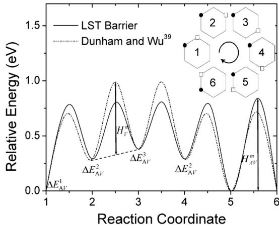
FIG. 1. (Color online) The idealized Dunham and Wu (Ref. 39) path compared to the path calculated by using LST simulations to estimate the migration energy of the  $V$  with respect to an As atom. The inset represents the ring mechanism of diffusion for the AsV pair (As=black circles and V=squares) projected onto the (111) surface of Ge.
