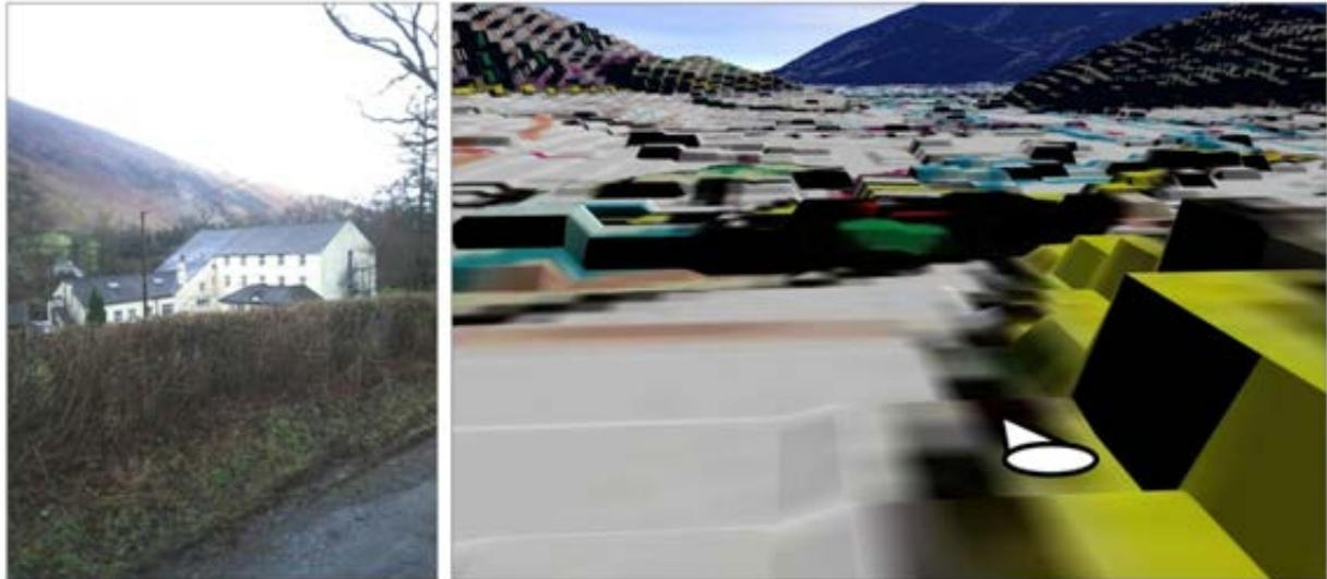
Figure 5. Example of the representational issues present with the DSM. The photograph (left) as taken from the location indicated in the 3D visualisation (right).
