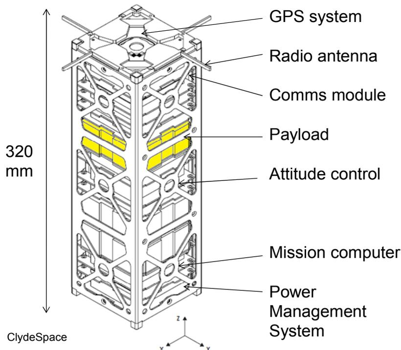
Figure 2: UKube-1 structure showing the outer Pumpkin space frame. A single instrument payload slot is highlighted (source: ClydeSpace<sup>6</sup>).
