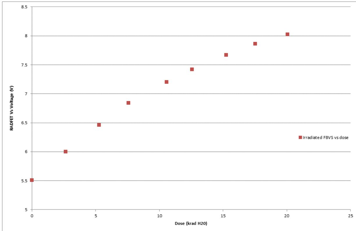
Figure 6: RADFET Flat Band Voltage Shift (FBVS) measured as a function of dose.
