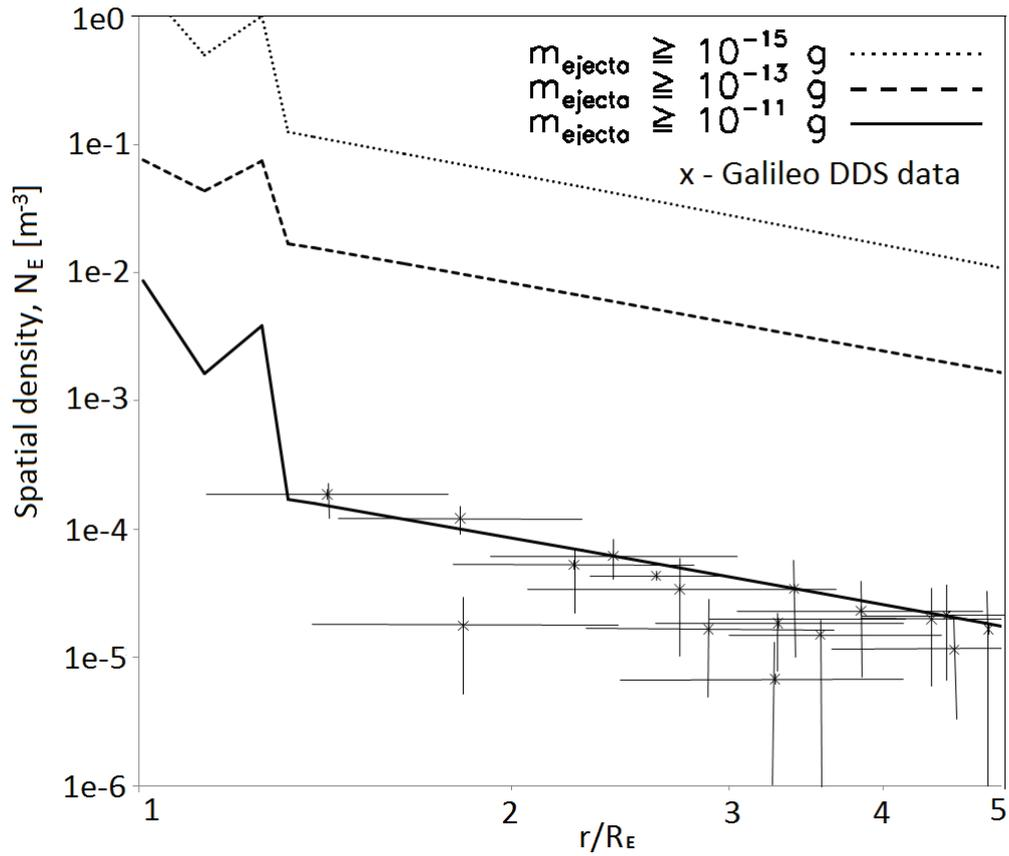
Figure 9: Radial spatial density of ejecta from Europa (measured from the centre of the moon), for dust masses larger than three different mass thresholds ( $10^{-15}$  g,  $10^{-13}$  g and  $10^{-11}$  g), compared with Galileo data. Galileo DDS had a detection mass threshold at  $10^{-11}$  g for this set of data (Grün et al., 1992), which matches our model predictions.
