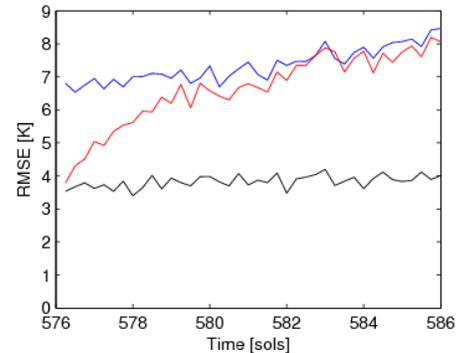
**Figure 3:** Global mean RMSE [K] to TES observations from a freely running model (blue), atmospheric reanalysis (black), and forecast initialized from a reanalysis (red) using an ensemble data assimilation system [3], demonstrating the capability for Mars numerical weather prediction.
