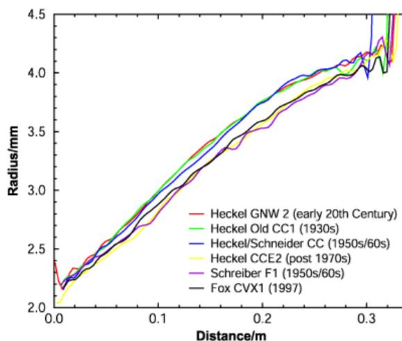
Figure 1: Bore profiles of six bassoon crooks.
