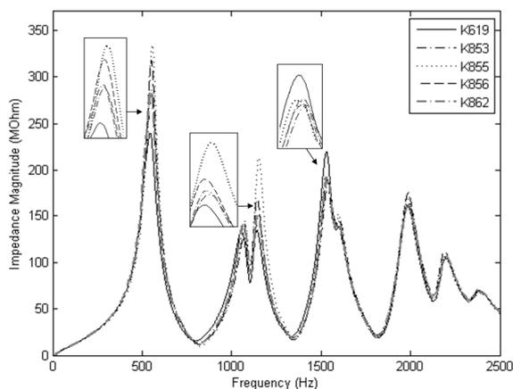
Figure 2: Input impedance magnitude curves for five Howarth student model oboes with F6 fingering applied.
