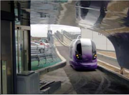
Fig 5: A Heathrow PRT 'pod' descending from the elevated guideway to a car park station
