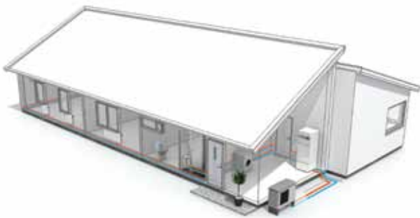
Air source heat pump
