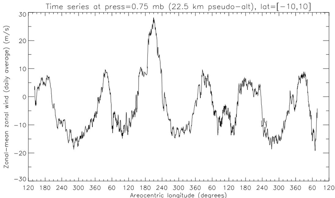
Figure 2, time series of the zonal-mean zonal wind in the latitude band  $[-10, 10]$  degrees at 0.75mb (corresponding to a pseudo-altitude of 22.5 km)
