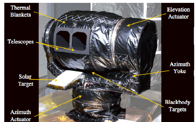
Figure 1 – The MRO/MCS instrument during thermal vacuum testing at JPL
