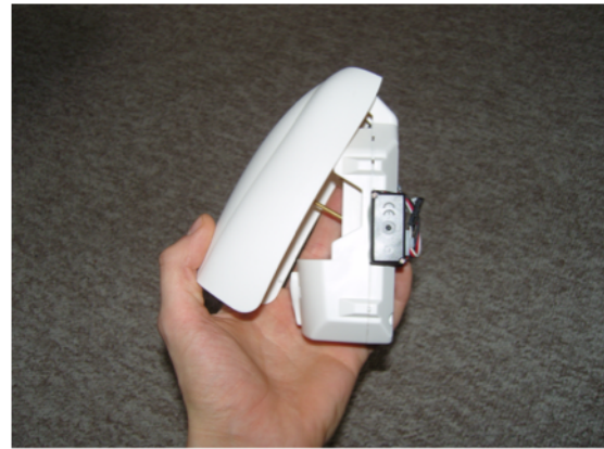
Figure 1. The first prototype for the sensory augmentation device using an air freshener case shown in its opened state
