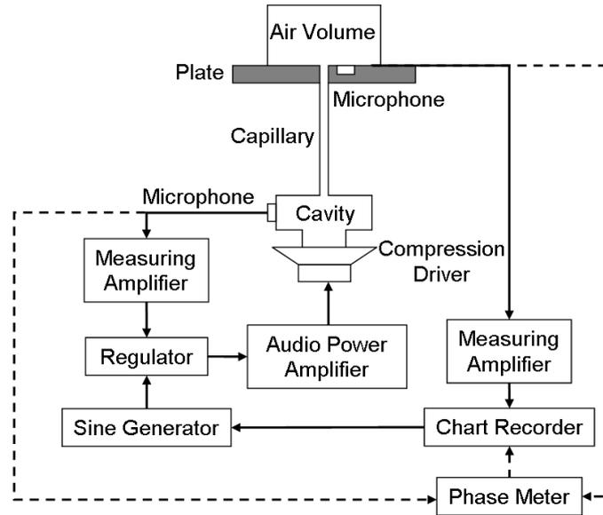
Figure 1 Dual microphone capillary-based impedance measurement set-up.
