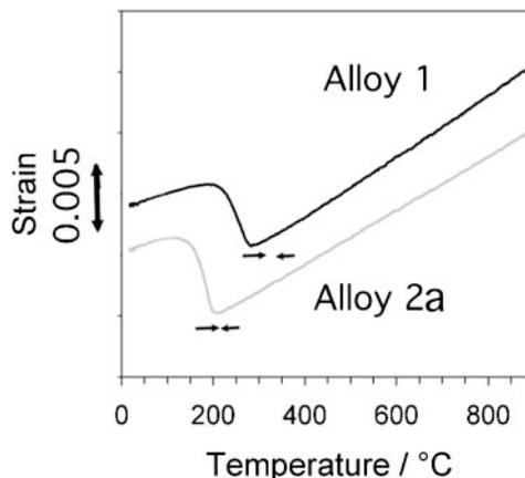
6 Dilatometric data: arrows indicate 95% confidence limits in determination of  $M_s$  temperature; for alloy 1,  $M_s$  is determined to be  $327 \pm 13^\circ\text{C}$  and for alloy 2a,  $216 \pm 2^\circ\text{C}$
