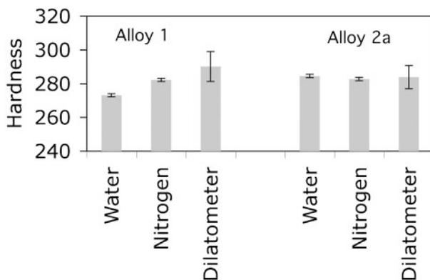
5 Vickers hardness (10 kg) measured on samples which were water quenched, quenched in liquid nitrogen and cooled in a dilatometer at 10 K s<sup>-1</sup>; error bars represent range of measurements; notice exaggerated scale; differences in hardness between different samples are small
