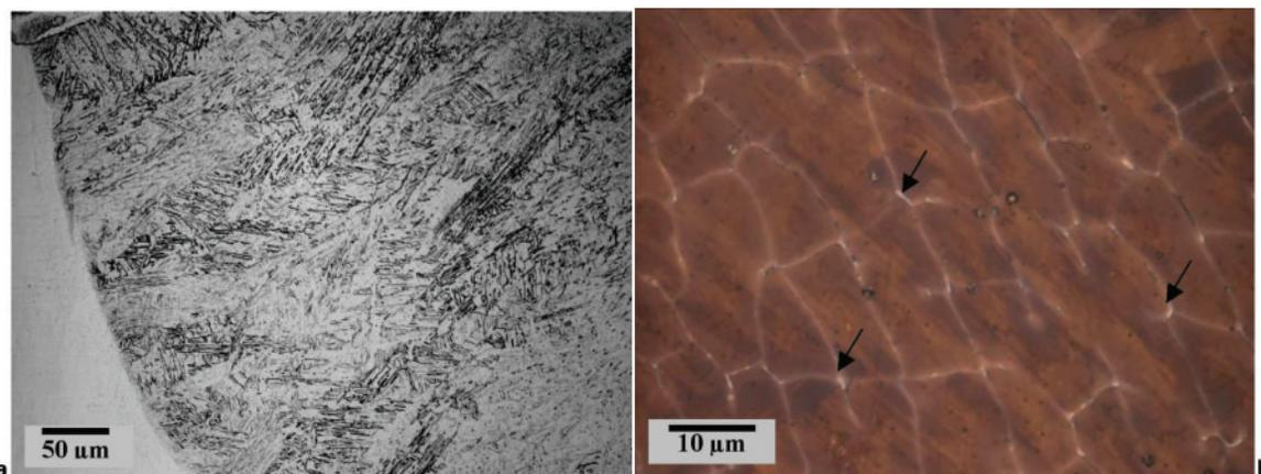
a essentially martensitic microstructure revealed by etching with Fry's reagent; b high magnification image showing small amount of discontinuous  $\delta$  ferrite revealed by using Lichtenegger colour etching
