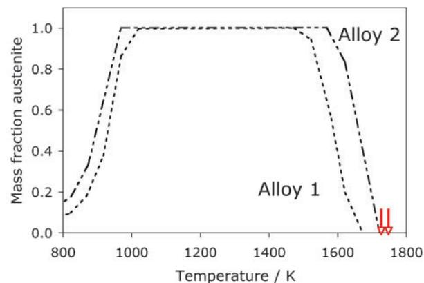
3 Calculated austenite content of alloy 1 (0.01C-12.9Cr-4Ni-1.5Mn, wt-%) and alloy 2a (0.01C-13Cr-6.12Ni-1.2Mn, wt-%): full compositions are listed in Table 1; two arrows on right are solidus temperatures, 1750 and 1730 for alloys 1 and 2a respectively
